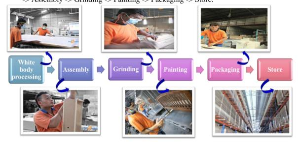
The main production process of the company's kitchen cabinet products is divided into 7 major processes, as shown in the following figure: White Body Processing -> UV Roller Coating -> Assembly -> Sanding -> Painting -> Packaging -> Store.
